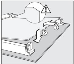
Replace the first of the middle panes. Make sure the cut-off corner is positioned at the top right hand side.
